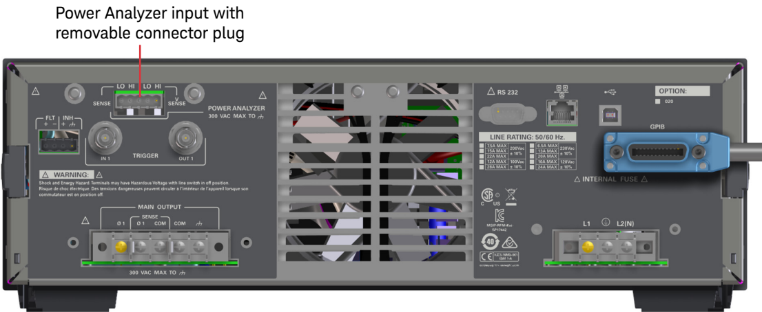
Figure E-2 Rear panel - overall view
