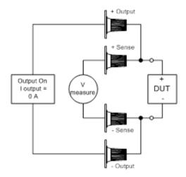
**Current Measure** - the Current Measure selection emulates a zero-burden ammeter. Voltage priority mode is set by default. The +/- Current Limits are set to their maximum values. The current measurement cannot exceed the current ratings of the unit as indicated in the +/- Current Limit fields.
