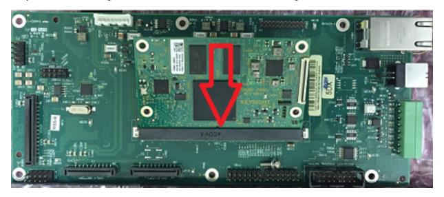
**Step 5.** Then position the heat spreader over the board and gently push the heat spreader down. Install the four screws.
