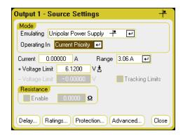
Resistance - This is only available on Keysight N6781A and N6785A. Output resistance programming is primarily used in battery emulation applications, and only applies in Voltage Priority mode. Values are programmed in Ohms, from – 40 m $\Omega$  to + 1  $\Omega$ .
