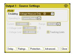
**Voltage Measure** - the Voltage Measure mode works best when the sense terminals are connected to the output terminals. You can use 4 Wire sensing and connect the sense and output leads directly to the DUT as shown below, or you can use Local sensing and connect only the output leads to the DUT.
