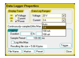
Some models have a high measurement range labeled CComp On, which is selected by default. The CComp On range compensates output current measurements during voltage transients. For more information, see **Dynamic Current Measurement Control**.
