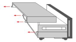
Step 2. Place the power modules in the mainframe.
