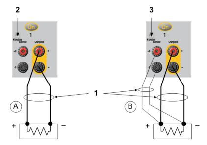
Connect the load to the output terminals using separate connecting wires. Keep the wire-pair as short as possible and twist or bundle it to reduce lead inductance and noise pickup. Keep the load leads under 14.7 meters (50 feet) per lead because of inductance effects.
