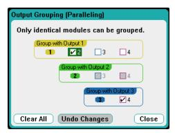
Grouped outputs are controlled using the output number of the **lowest** output in the group. As shown in the following figure, output 1 is grouped with output 2 and output 3 is grouped with output 4.
