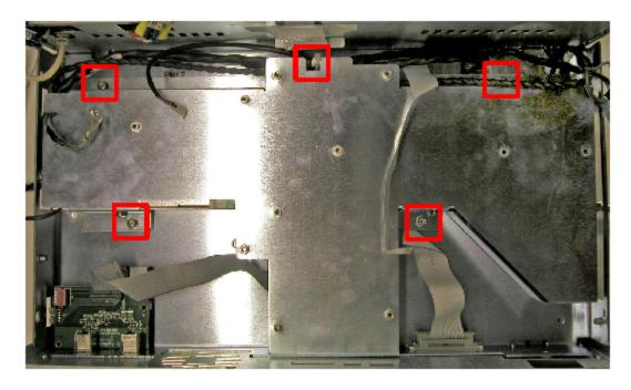
**Step 4.** Remove four screws using a T20 driver from the sides of the bulk shroud and remove the bulk shroud.
