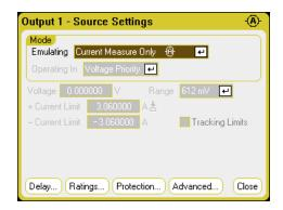
The following additional settings are also required. Remote sensing (4 Wire) is always required. For applications with transient voltage drops, use the High3 setting with a compensation capacitor across the DUT. Capacitors can be film or ceramic with values from 7  $\mu$ F to 150  $\mu$ F. Refer to Keysight N678xA SMU Wiring for additional wiring information.
