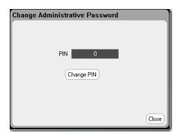
If the password is lost or forgotten, access to the Administrative Tools menu can be restored by setting an internal switch to reset the password to 0. If the message "Locked out by internal switch setting" or "Calibration is inhibited by switch setting" appears, the internal switch is set to prevent the password from being changed (refer to the calibration switches section).
