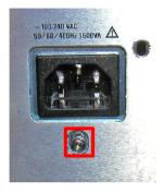
**Step 3.** Disconnect the two connections and remove two screws using a T20 driver from the AC Module.
