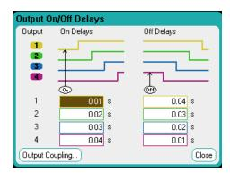
All power modules have an internal turn-on delay that applies from the time that the command to turn on the output is received until the output actually turns on. This turn-on delay is automatically added to the On Delays values. The turn-on delay does not apply when outputs turn off. To view the delay, select the Output Coupling button.
