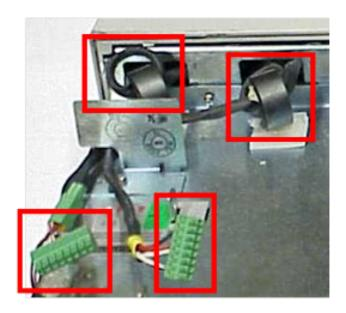
**Step 7.** To install the top chassis, perform steps 1-6 in reverse order. Be sure to tuck all cables in before replacing the top chassis
