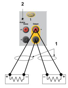
This minimizes mutual coupling effects and takes full advantage of the power module's low output impedance. Keep each wire-pair as short as possible and twist or bundle the wires to reduce lead inductance and noise pickup. The goal is to always minimize the loop area or physical space between the + and - load wires from the power analyzer to the load. Keep the load leads under 14.7 meters (50 feet) per lead because of inductance effects
