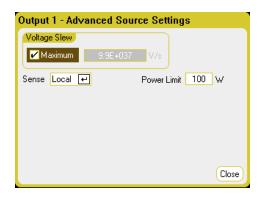
For Keysight N6705 mainframes, the instrument will operate normally as long as the combined output power is within the power rating of the mainframe If the combined power drawn from all of the outputs exceeds the mainframe's power rating of 600 W, a power fault protection event will occur. This causes ALL outputs to turn off and remain off until a protection clear command is given. A status bit (PF) will indicate that a power fault protection event has occurred.
