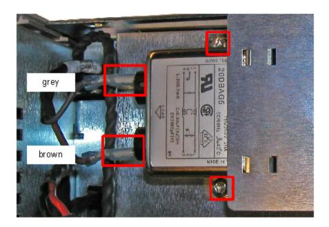
Step 4. Remove the AC Module
