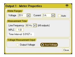
The instrument will continuously display the auxiliary voltage measurement on the front panel Meter View.
