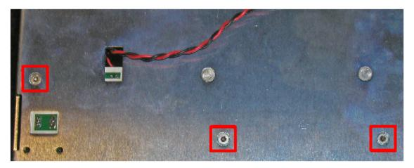
**Step 3.** Disconnect any remaining cables if required, and either cut or carefully slide the two push-on retainers off of the retaining pins.
