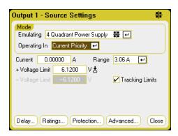
Operating in – selects either Voltage Priority or Current Priority. In voltage priority the output is controlled by a bi-polar constant voltage feedback loop, which maintains the output voltage at its positive or negative setting. In current priority the output is controlled by a bi-polar constant current feedback loop, which maintains the output source or sink current at its programmed setting. Refer to N678xA Multi-Quadrant Operation for a detailed description of voltage and current priority.
