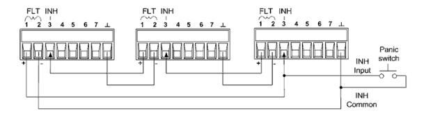
As shown in the figure, when the Fault outputs and Inhibit inputs of several instruments are daisy-chained, an internal fault condition in one of the units will disable all outputs without intervention by either the controller or external circuitry. Note that when using the Fault/Inhibit signals in this manner, both signals must be set to the same polarity.
