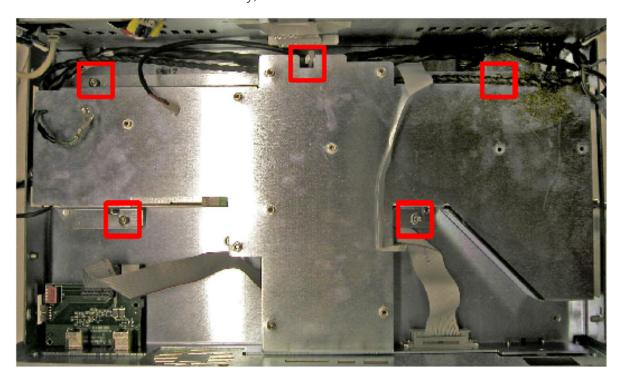
**Step 6.** Gently lift bulk shroud out of mainframe and place on right side of mainframe (non-handle side - right side when viewed from front).
