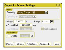
Battery Emulator - lets you specify the battery voltage and range as well as the + and - current limits. The output resistance is programmable, from – 40 m $\Omega$  to + 1  $\Omega$ . Voltage Priority mode is locked. The voltage setting is limited to positive values. The + and - current limits are set to their maximum values. The – current limit setting sets the current limit when the battery is being charged.
