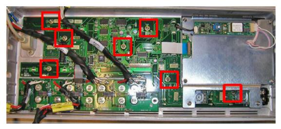
**Step 4.** Remove the seven knobs from the front panel.
