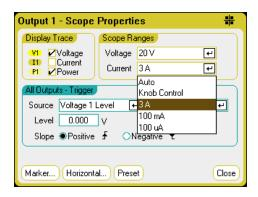
Selecting Knob Control allows the Vertical Volts/Div knob on the front panel to automatically select lower measurement ranges at higher measurement resolutions. For lower measurement resolution a higher range is automatically selected. The present range is displayed on the lower left corner of the Scope View window.
