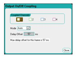
Normally, the firmware automatically calculates the delay offset based on the longest minimum turnon delay of the installed power modules. However, if you will be excluding some outputs from participating in an output on/off delay sequence as described Step 3, the delay offset may be different based on the outputs that you will actually be sequencing. The minimum turn-on delays of the power modules are documented in the **Keysight N6700 DC Power Analyzer Family Specifications Guide**.
