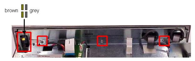
**Step 6.** Remove two screws using a T10 from each side of the front panel.
