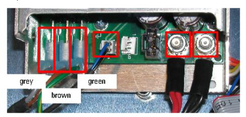
Step 6. Remove the bulk supply.
