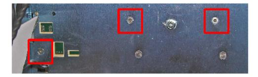
**Step 8.** Disconnect any remaining cables if required, and either cut or carefully slide the two push-on retainers off of the retaining pins.
