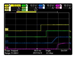
Note that the delay for output 1 does not start until 57 milliseconds have elapsed. This is because the internal delay for the mainframe used in this example is 57 milliseconds. This built in delay precedes any user-defined delays that have been programmed.
