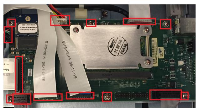
Step 3. Remove the Processor Carrier by sliding forward and lifting.
