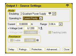
Operating in – selects either Voltage Priority or Current Priority. The other settings in 2-quadrant mode are the same as the settings in 4-quadrant mode except that you cannot program negative voltages or negative voltage limits. Because of this, voltage tracking is not available in Current Priority mode. Note that the negative voltage limit is fixed at –10 mV. Refer to N678xA Multi-Quadrant Operation for a detailed description of voltage and current priority.
