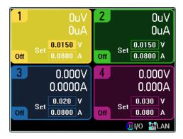
Press one of the four On keys to enable an individual output. In Meter View the power analyzer continuously measures and displays the output voltage and current of each output.
