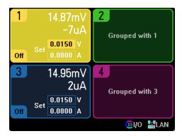
To return grouped outputs back to an ungrouped state, turn the output off and remove the parallel connections between the outputs. Then uncheck the check boxes. Then cycle AC power to the unit for the grouping or ungrouping changes to take effect. Grouped settings are saved in non-volatile memory.
