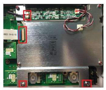
**Step 3.** Disconnect one cable and remove four screws using a T10 driver to remove display from bracket.
