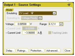
**CC load** - lets you specify the input Current and Range as well as the + Voltage Limit. Current Priority mode is locked. Remember to set the input current to a negative value. The + Voltage Limit should normally be set to its maximum value. The - Voltage limit is not programmable. In Meter mode, the measurement polarities and current settings are shown as negative values.
