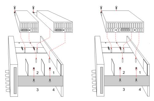
The location of the power modules inside the mainframe determines their front panel output and programming channel assignments. For example, modules installed in channel 1 will be connected to the wire harness for output 1. Modules installed in channel 4 will be connected to the wire harness for output 4.
