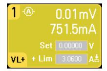
When the Measure Only modes are selected, the output is enabled and the voltage or current measurement is continuously displayed on the Meter View. Both voltage and current meters are active in either mode.
