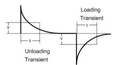
**Step 7.** The output voltage should return to within the specified voltage at the specified time following the 50% load change. Check both loading and unloading transient by triggering on the positive and negative slope. Record the voltage at time "t" in the performance test record form under "Transient Response".
