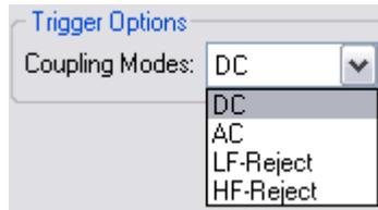
**DC coupling** allows DC and AC signals into the trigger path. When DC coupling is selected, both DC and AC components of the input waveform are transferred to the oscilloscope. DC coupling enables the triggering waveforms of as low as 0 Hz without large DC offsets to be captured.
