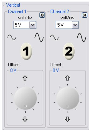
**Figure 2-1** Soft front panel vertical system controls
