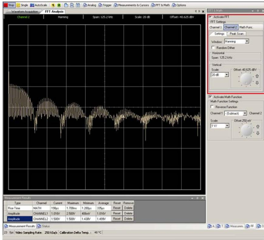
Figure 2-12 Waveform obtained with Hanning window selected
