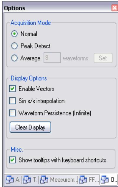
**Figure 2-16** Soft front panel of the Options Controls
