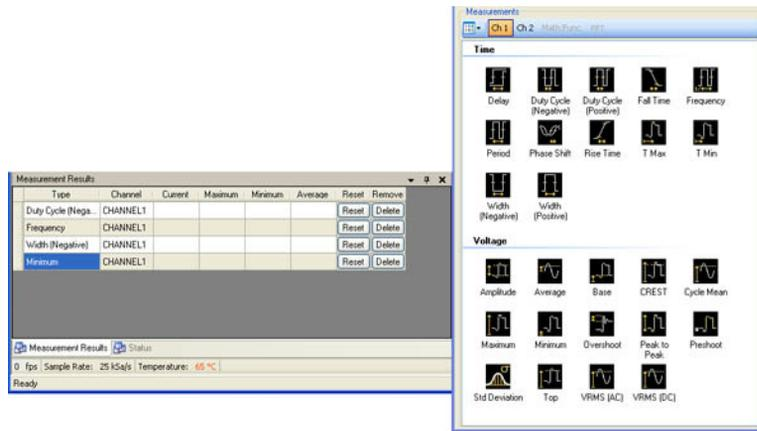
**Figure 2-9** Measurements panel and Measurements Results panel
