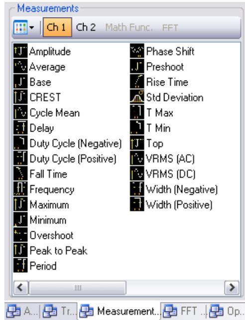
**Figure 2-8** Automatic measurements on the Measurements & Cursors panel
