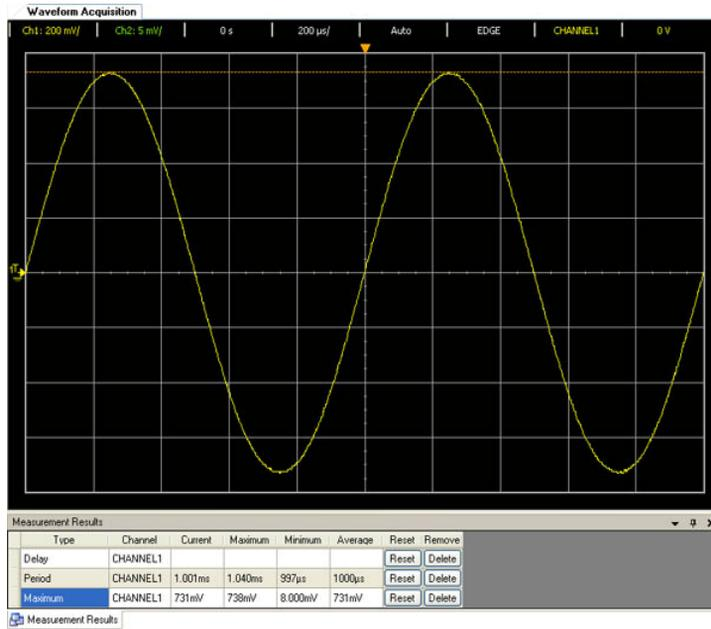
**Figure 2-7** Auto marker automatically marks the maximum value of the waveform when Maximum measurement is selected
