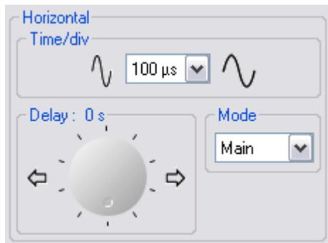
**Figure 2-4** Soft front panel horizontal system controls
